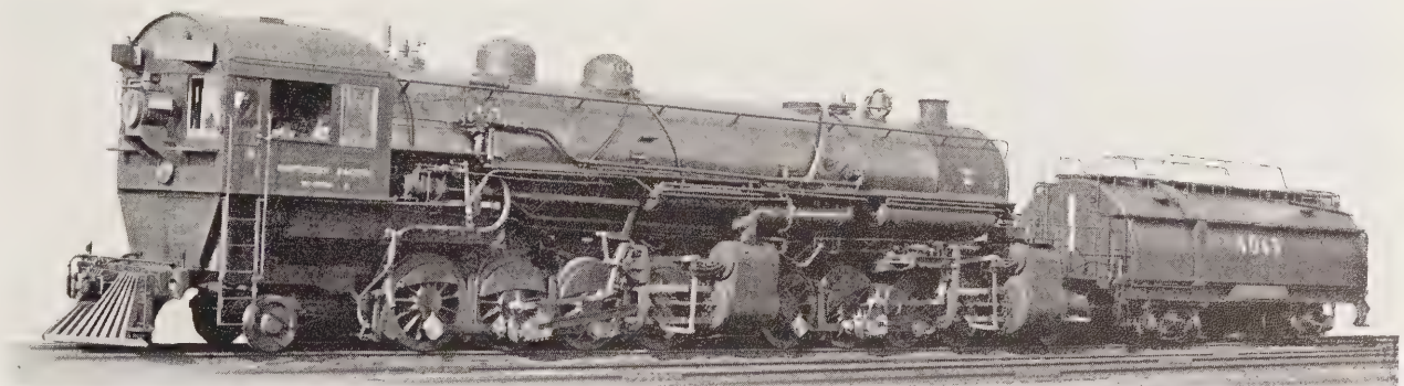
A Mallet Locomotive of the 2-8-8-2 Type, Built by The Baldwin Locomotive Works in 1912
